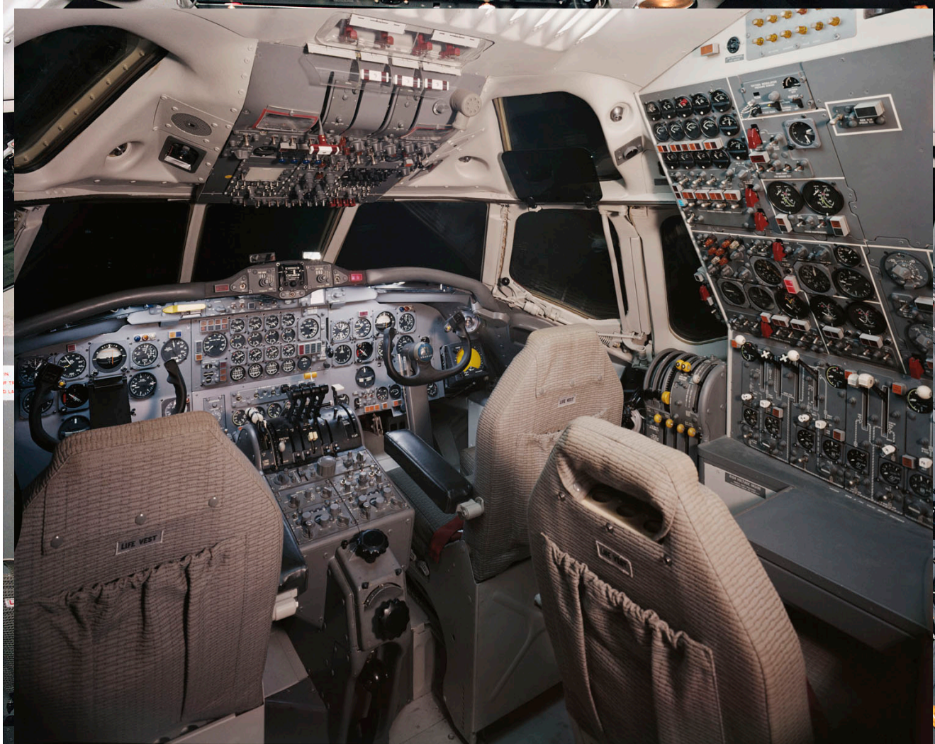
747-200 Flight Deck A thousand lights, gauges & switches
